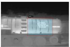
One of the key features of our dual camera system is its ability to check the truck's internal level. This allows you to see if there is an oil interface inside the truck. By monitoring these levels, you can quickly identify any deviations from standard procedures and take immediate action, if necessary.
